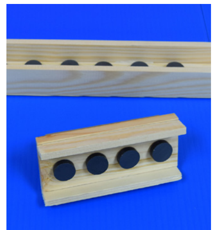
Figure 12 - Maglev train underside showing position of magnets.
