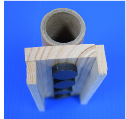
Figure 11 - Maglev Train model showing position of the pieces of wood and magnets.
