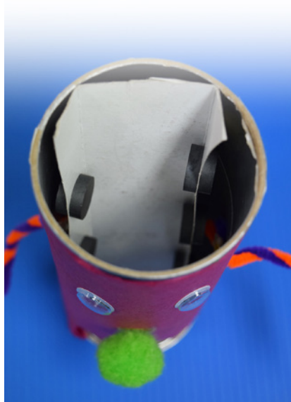
Figure 2 - Inside the model - showing the magnets positioned on the cardboard chute.
