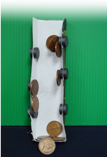
Figure 3 - Cardboard chute showing magnetic and non-magnetic coins.
