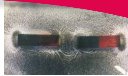
Figure 11b - Iron filings show field line around 2 magnets with opposite poles facing.
