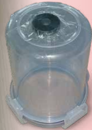
Figure 4 - Magnet secured to underside of one container using tape.
