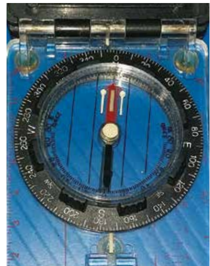
Figure 12 - Compass with red needle pointing north and black needle pointing south.
