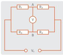
Figure 1 – Wheatstone Bridge circuit.
