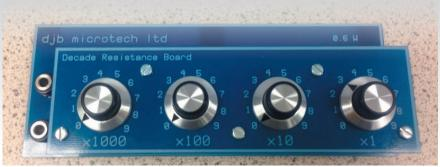
Figure 3 - calibrated variable resistor.
