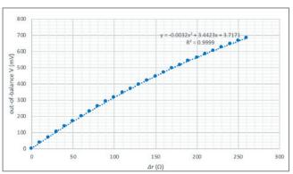
Figure 5 - Out-of-balance V versus Δr with larger Δr.
