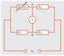
Figure 2 - Unbalanced Wheatstone Bridge.
