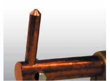
Figure 6 - Electrode angle.
