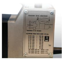
Figure 3 - Weld pressure forces.
