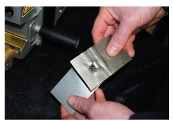
Figure 10 - Testing weld quality.
