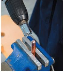
Figure 8 - Electrode cutter fixed into drill chuck.
