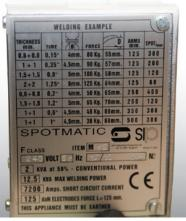
Figure 5 - Welding times.
