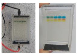
**Figure 4**: Electrophoresis tank set up with carbon fibre electrodes, each connected to the power supply. 10  $\mu$ l of each sample are loaded into the wells. Electrophoresis should continue at 36 V for 20 minutes. The result shown on the right could be used to demonstrate that Suspect 1 (well 2) matches the "DNA" sample obtained from the crime scene (well 1). Alternatively, akin to the original "Wizard Genes" protocol, the gel results could be used to determine the powers of each wizard.
