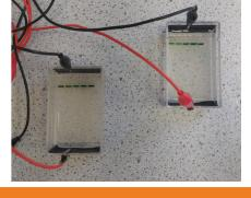
Remove the water from the prepared gel and replace with about 12 – 15 cm<sup>3</sup> sodium hydrogencarbonate buffer.
