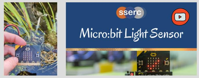
In the video above, you will see the Micro:bit used as a light sensor. Notice the "graphical" display changing as light levels alter; the numerical displays read 191, 63 and 105 (note down the values scroll across the screen).
