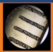
For this microscope: (40/400)x4 = <u>0.4mm diameter at</u> <u>x400</u> <u>magnification</u>
