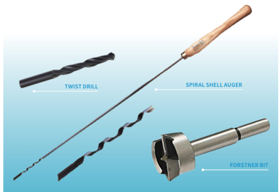
Figure 10 - Selection of boring tools.
