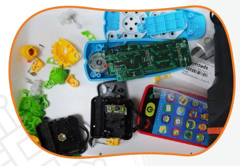
Some equipment enclosures are of a snap-fit design, which often requires leverage with some force. Avoiding this type of item is safer due to risks from prising open the snap-fit cover. Instead, use items which can be unscrewed or opened without excessive force.
