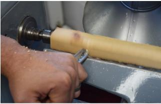
Figure 3 - Gouge tool position.
