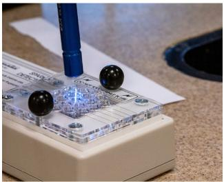
Figure 2 - The spark counter in action.
