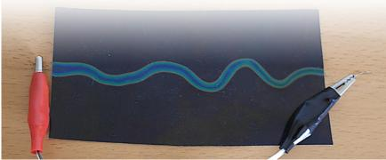
Figure 4 - Current causes heating.
