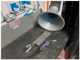
Figure 1 - Welding booth showing movable extraction arm/hood.
