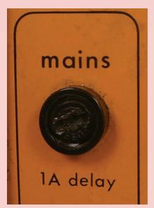
Figure 4 - Well-designed mains fuse holder.
