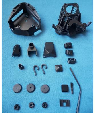
Figure 5 - 3D printed parts.
