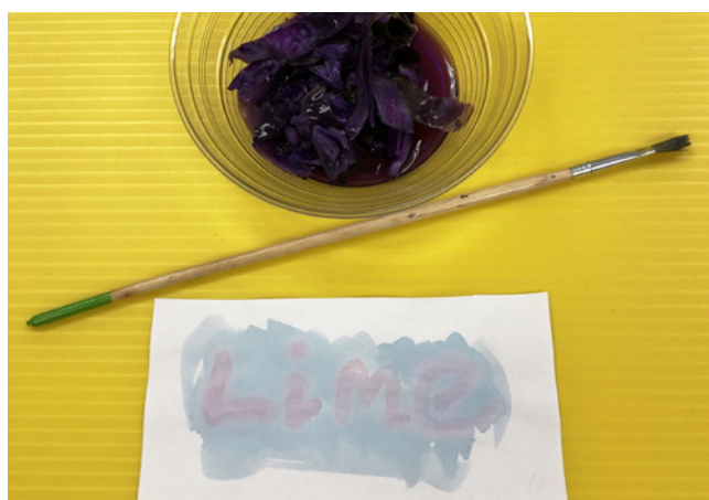
Figure 10 - Message written in lime juice revealed using red cabbage indicator.
