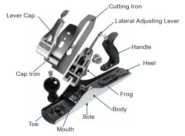
8.4.1 **Cutting Iron/Blade** – This is normally set to 45° to the sole of the plane. It is
