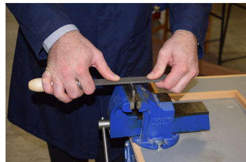
Right position - Work-piece set low in vice to provide maximum support.
