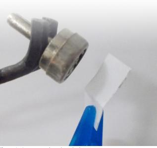
Figure 1 - A source undergoing a leak test.
