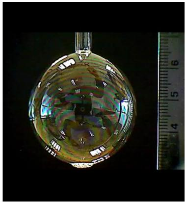
The bubble was susceptible to bursting due to air currents, so we lowered it into a glass beaker to protect it.
