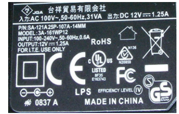
Figure 1 - Markings on a branded power supply. The GS Mark shows that the product has been independently tested for conformance with safety standards.
