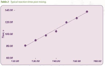
*Figure 2* - Time taken, as a function of volume of water, for the appearance of the characteristic bue colour of iodine-starch complex. Experimental details in the text.
