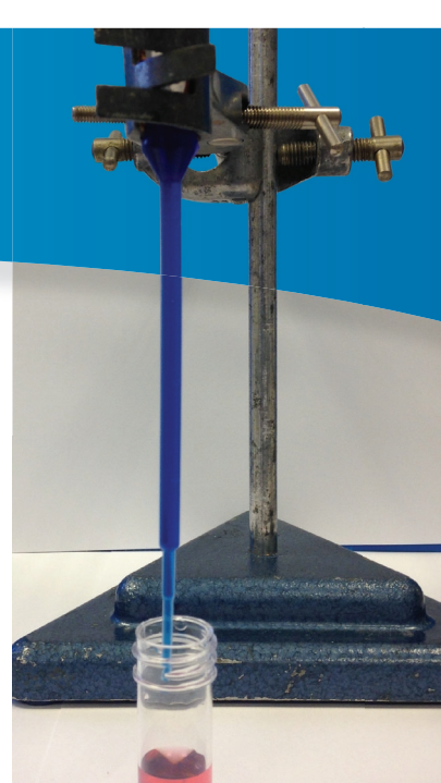
Figure 5 - Micro-titration using drops from a Pasteur pipette.
