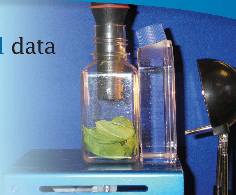
Figure 1 - Experimental set-up for measuring respiration and photosynthesis rates in plants. Basil leaves (ca. 5 g) are placed into a 'reaction chamber' together with a CO 2 gas sensor (Product code VR105512) from Instruments Direct Services Ltd. The sensor is linked to a computer via a Vernier Go!Link interface. Data were collected at 4 second intervals for some 9000 s with the lamp being switched on during the periods 360-1300 s, 2040-2912 s, 3860-4680 s, 5740-6760 s, and 7928-8796 s. At other times the apparatus was in darkness. Plots of data are shown in Figures 2 and 3.
