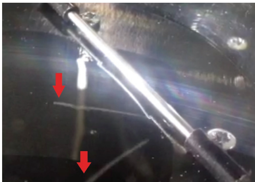
Figure 2 - Tracks in a cloud chamber.
