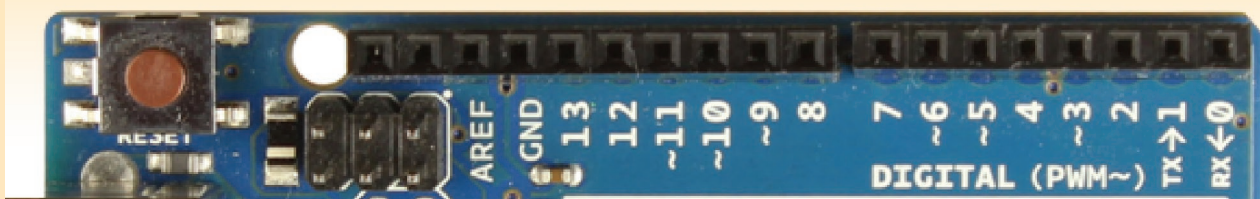
Figure 3 - Digital connections on the Arduino UNO Board.
