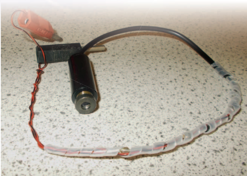
Figure 1 - The violet LDM with chain of diodes.
