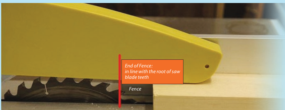
Figure 3 - Correct Fence Setting to Prevent Kickback- taken from the Poster.
