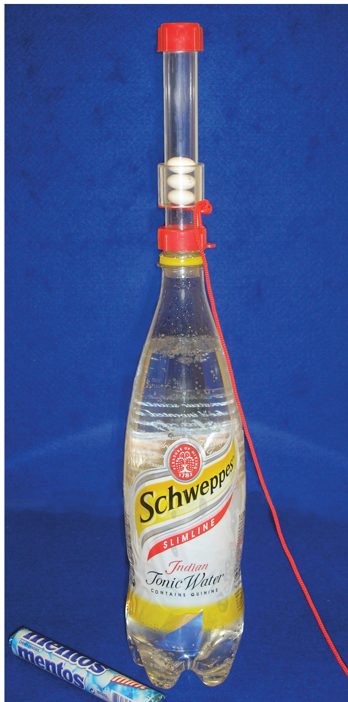
Figure 1 - Geyser Tube arrangement with 3 Mentos™ in place. Removal of the pin (located just underneath the Mentos™) releases the Mentos™ into the bottle.
