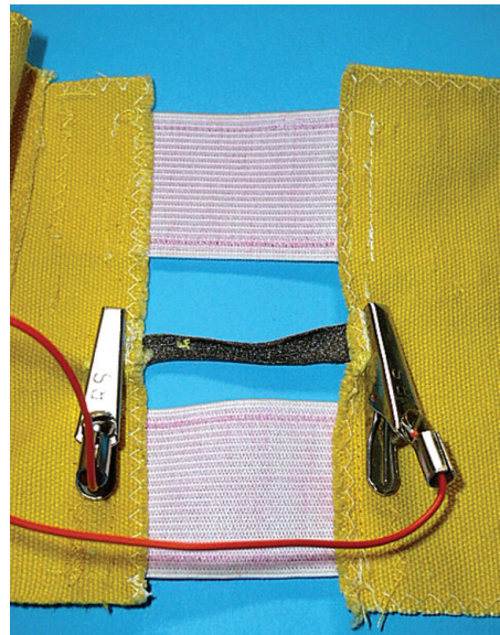
Figure 3 - Insert one jaw of the croc clip through the buttonhole.
