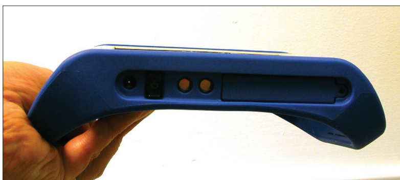
Figure 2 - on/off switch and charging sockets (base of unit).
