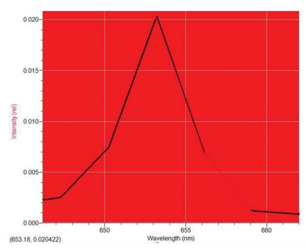
Figure 14 - Spectrum from laser diode module (SpectroVis).
