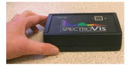
Figure 1 - SpectroVis spectrophotometer.
