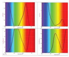
*Figure 7* - *Absorbance (top) and transmittance graphs for two dyes.*
