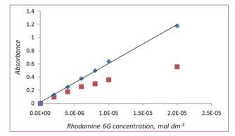
**Figure 5** - Absorbance as a function of the concentration of aqueous solutions of rhodamine 6G. Excitation was 535 nm and pathlength was 1 cm. The colorimeter used was either a CO7500 colorimeter using a 520 nm filter ( $\blacklozenge$ ) or the Mystrica Colorimeter ( $\blacksquare$ ).
