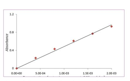
**Figure 9** - Absorbance, as measured using the Mystrica Colorimeter, as a function of the concentration of aqueous solutions of methylene blue. Pathlength was 1 cm.
