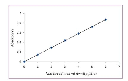
*Figure 3* - Absorbance, as measured using the Mystrica Colorimeter, as a function of the number of neutral density filters present. Each neutral density filter is rated by the manufacturer as having an absorbance of 0.3. Excitation wavelength was 535 nm.
