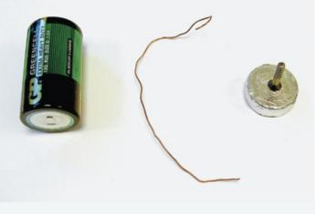
Figure 1 - Basic parts of a homopolar motor
