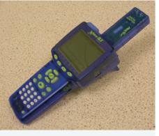
Figure 3 - Xplorer and digital adapter
