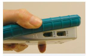
Figure 9 - Labquest digital ports
