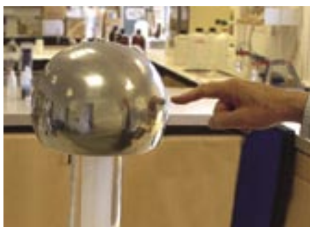
Figure 3 - Corona discharge through a projecting finger.
