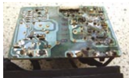
Figure 4 - Track-side view of a plug-top power supply damaged by a VDG spark.
