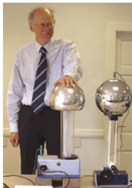
Figure 2 - Determining the voltage on a dome when charging a person.
