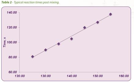
*Figure 2* - Time taken, as a function of volume of water, for the appearance of the characteristic bue colour of iodine-starch complex. Experimental details in the text.
