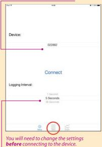
**Figure 4** - Connecting and setting sample times with the iOS app.
