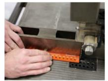
Figure 3 - A 20 mm accurate thickness gauge.
