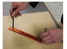
Figure 4 - Diameter/radius marking holes.
