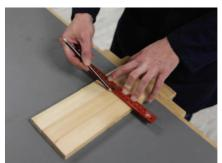
Figure 5 - Accurate straight edges for marking out.
