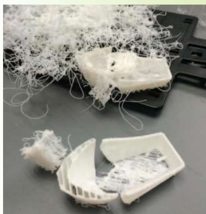
Figure 5 - The support material blockage results.
