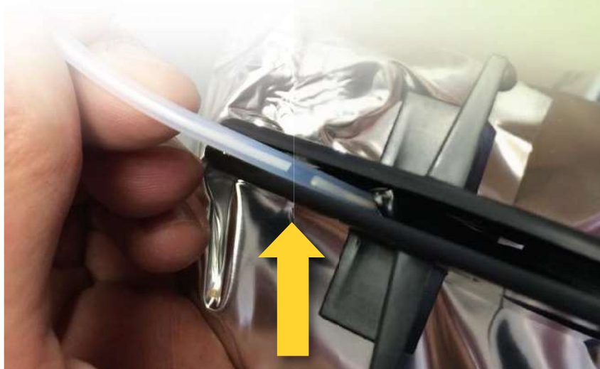
Figure 6 - The breakage in the support material supply.
