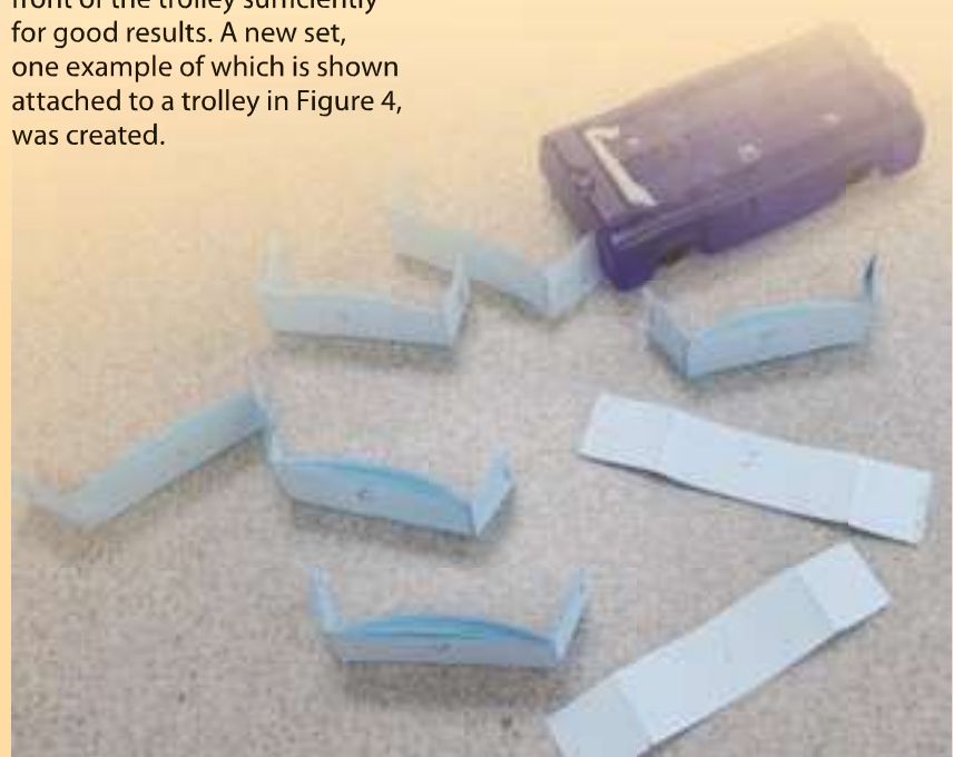
Figure 3 - Trolley with crumple zones of varying thickness.
