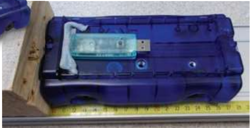
Figure 5 - Trolley with accelerometer.
