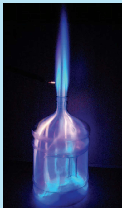
Figure 1 - Whoosh bottle with methanol.
