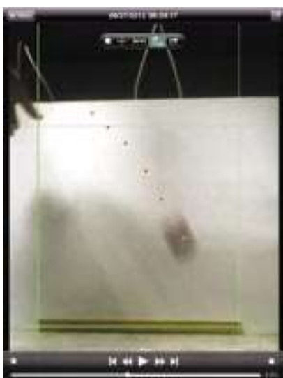
Figure 5 - a ball being tracked using Video Physics.
