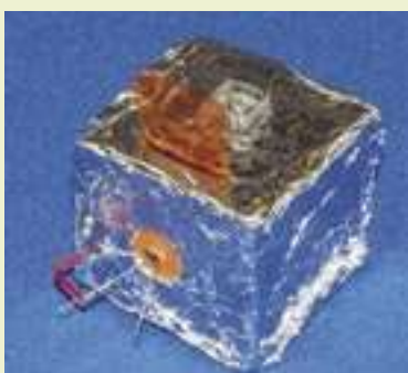
Figure 12 - Push the resistor into the block and connect to the LED with wire.
