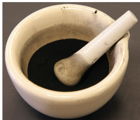
Figure 1 - Prepared ore containing activated charcoal and copper carbonate.
