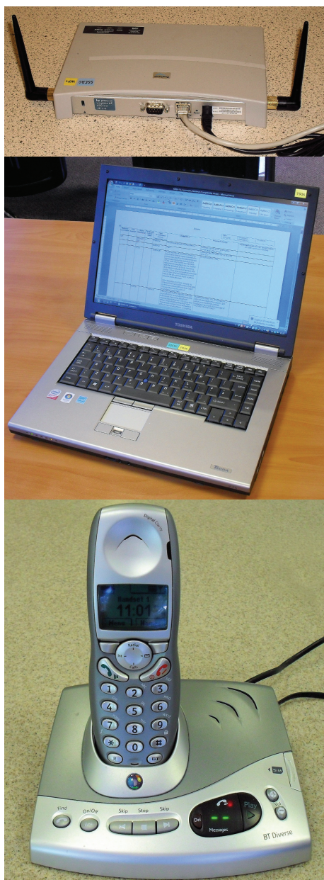
Figures 1a, b & c - Typical WiFi products: wireless router, laptop and digital enhanced cordless telecoms (DECT) phone.
