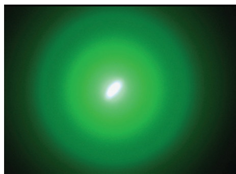
Figure 4 - Display from Electron Diffraction Tube.
