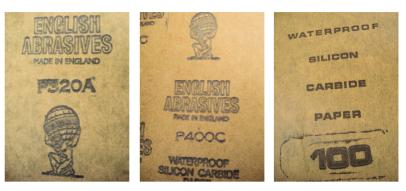
Figure 3 – Reverse of different types of abrasive sheets
