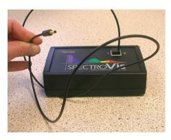
*Figure 2* - SpectroVis with optional optical fibre probe.
