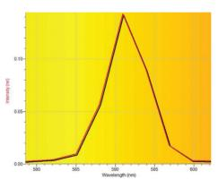
*Figure 4* - Zooming in on the sodium yellow line (SpectroVis).
