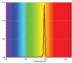
*Figure 3* - *Spectrum from sodium lamp (SpectroVis).*
