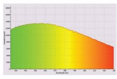
*Figure 13* - Sodium absorption spectrum. Note the wee nick in the spectrum at around 589 nm where most absorption takes place.
