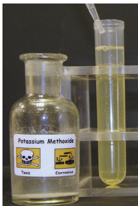
Figure 4 – Potassium methoxide is added to the vegetable oil using a pipette.
