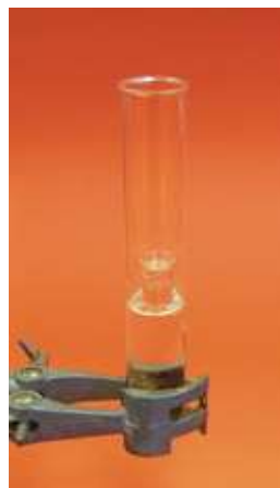
Figure 2: The small Pyrex test tube only becomes visible when some of the glycerol is poured away
