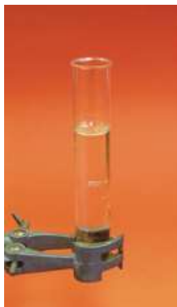
Figure 1: A small test tube almost invisible inside a larger tube of glycerol
