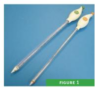
The graduated pipette part (called a syrette) (Figure 1) is coated with fluoro-plastic (FEP) and has a thread at the end. This screws into the diji hand-piece part (Figure 2) and can therefore reduce the potential for glass piercing injuries which can occur when attaching
