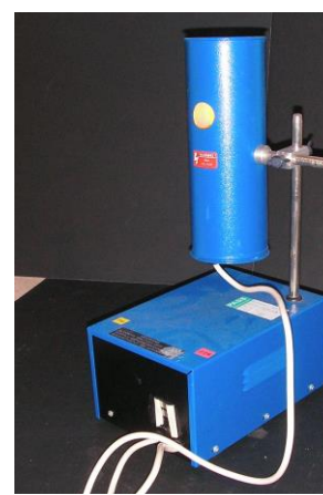
Figure 2 – Sodium lamp and power supply
