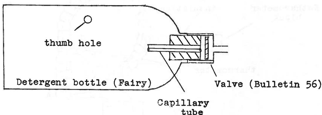
The capillary tubing ensures a slow stream of air when the hole is closed by the thumb and the detergent bottle pressed. Without this controlled flow of air there would be the danger of quick pressing giving a surge of air sufficient to blow any powder, etc. out of the reaction tube.
