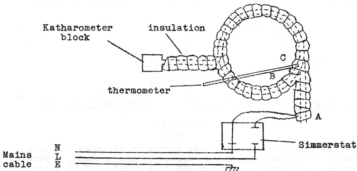
The connections on the regulator should be well insulated by tape or protected by a perforated plastic box placed over it.
